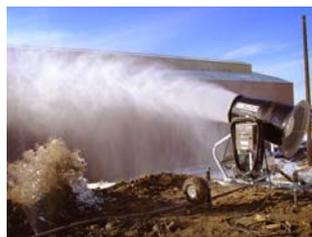
Picture from dustboss.com: environmental remediation dust control
