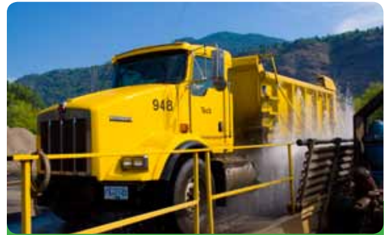
Wheel wash station at Trail Operations. Washing each truck leaving the storage area prevents metal-containing dirt from spreading along roadways on site, which in turn prevents dust going into the air.
