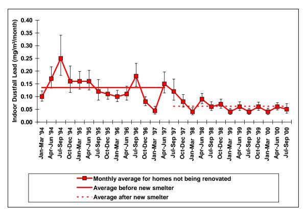
Figure 15 - Indoor Dustfall Lead Loading Before/After New Smelter
