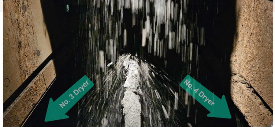
KIVCET feed mix being split between old and new dryers
